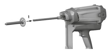
The fastener guide holds the insulation plug and in the driving process it directs the fastener to the desired position in the material.
